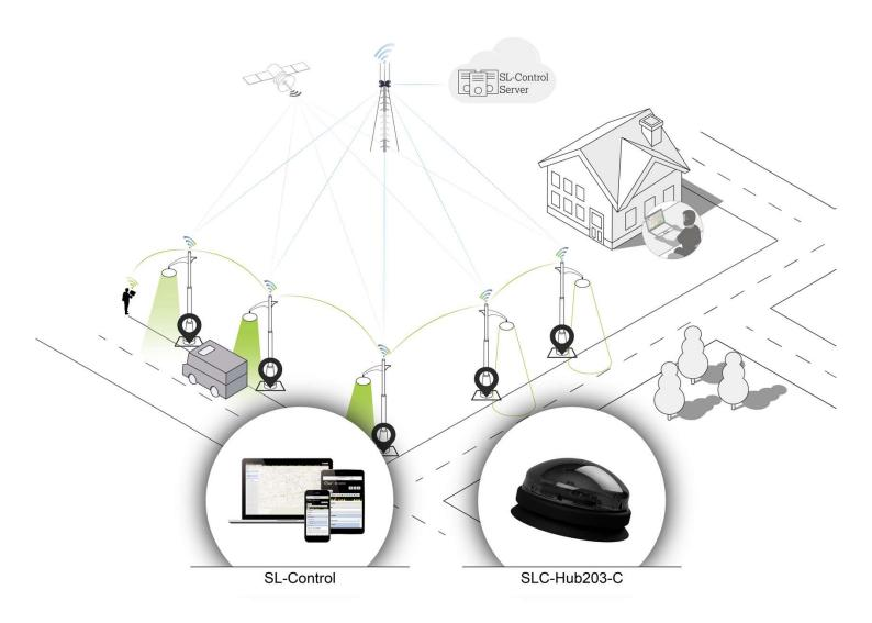
Thanks to the integrated eSIM and gateway function, an SLC-Hub203-C can establish a connection to the SL-Control web platform while maintaining a network with all other esave equipped lights within reach.
