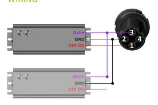
**Note:** The controller supports up to 4 LED Drivers simultaneously.
