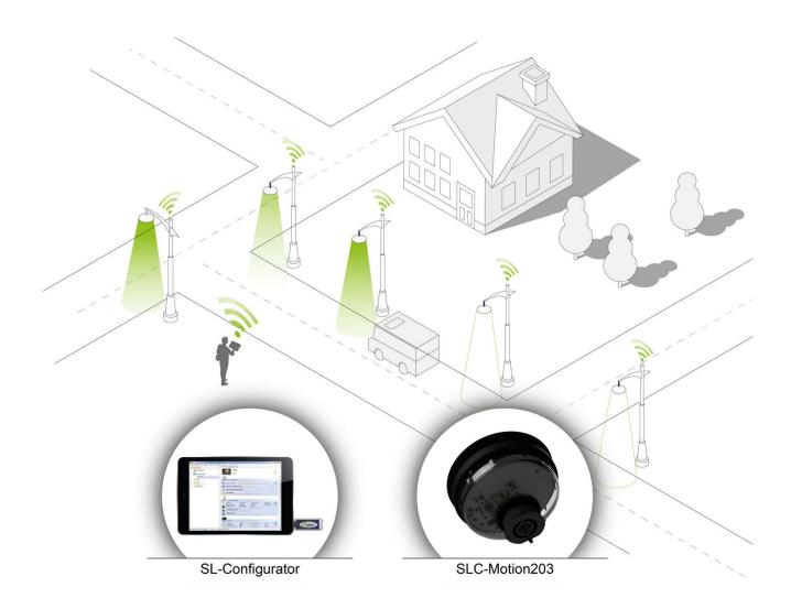
The Communication is ensured via an automatic, organizing 2.4 GHz mesh network. Each streetlight communicates with all luminaires which can be reached.
