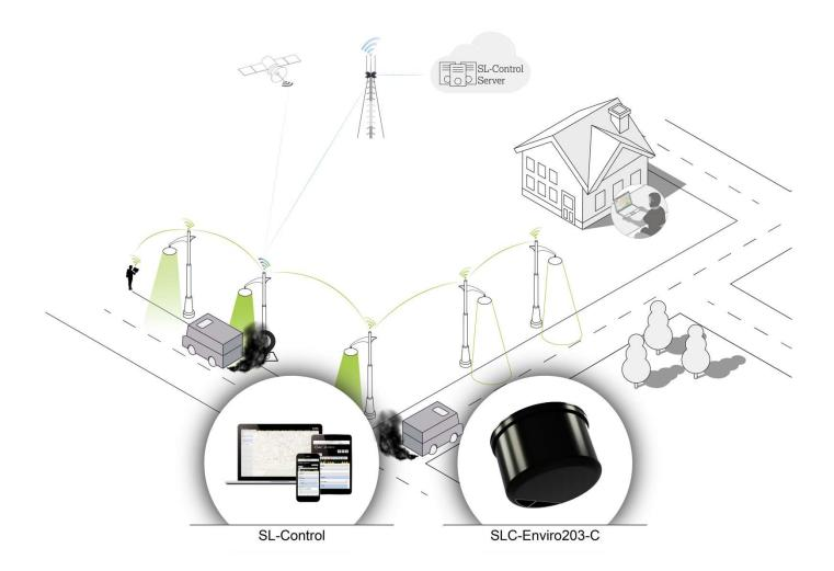
Thanks to the integrated eSIM and gateway function, an SLC-Enviro203-C can establish a connection to the SL-Control web platform while maintaining a network with all other esave equipped lights within reach.
